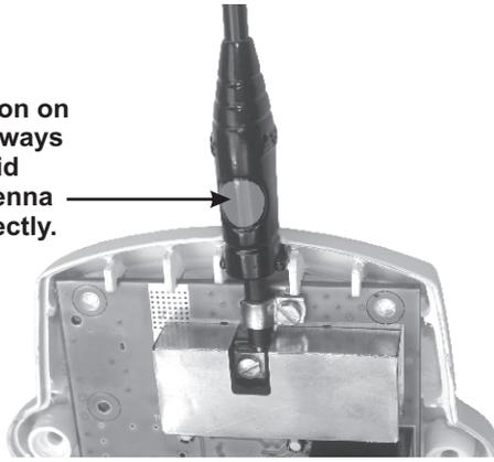
To install the antenna, slide it through the saddle and firmly into the square connector next to the screw. Tighten the square connector and saddle screws.
