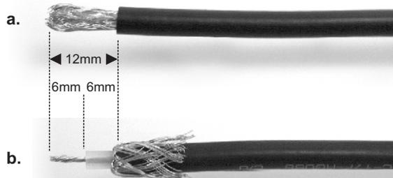
Fray and pull back the braiding and strip off 6mm of the inner white insulation leaving 6mm of the inner wire exposed.
