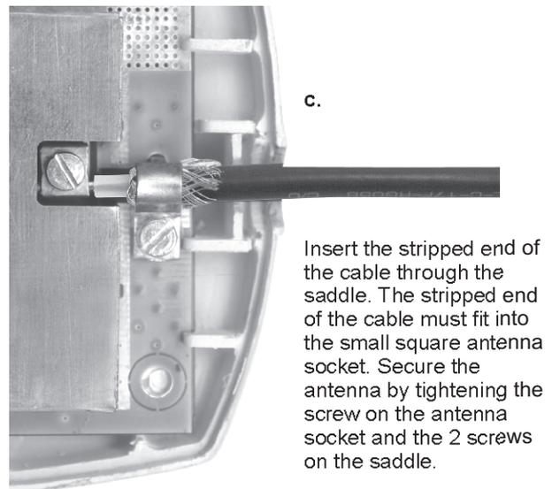
Insert the stripped end of the cable through the saddle. The stripped end of the cable must fit into the small square antenna socket. Secure the antenna by tightening the screw on the antenna socket and the 2 screws on the saddle.
